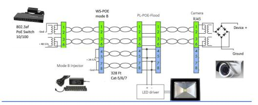
Your existing standard PoE switch supplies 48 or 56 volts DC for the device in mode A, and our PoE injector adds independent mode B power for the LED. Since these are on different pins of the RJ45 – it works well. With this method, our injectors from 1 to 24 ports are recommended for LED power on mode B, while a2<sup>nd</sup> device power comes from the PoE switch or injector on mode A pins.
