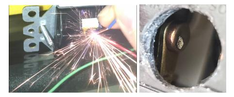
Sparks damage switches - 100 cycles and serious damage
